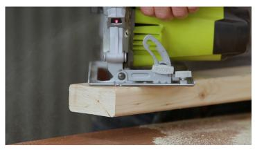
Cut the 2x4s. Clamp the 2x4s firmly to a work table and then use the circular saw to cut along the lines. A laser guide really helps.
