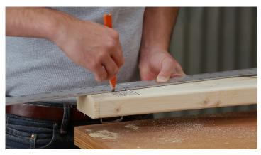
Mark the lines on the 2x4s. Measure and mark the 2x4s as shown in the diagram.
