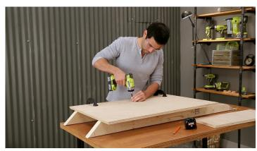
Glue and screw. Use wood glue and 2" screws to fasten the plywood panels to the 2x4s. Clamp the plywood in place or get a friend to help you position the plywood panels while you screw them. Use  $2\frac{1}{2}$ " screws to connect the 2x4 pieces to each other. Make sure to drive the screws into the plywood until the heads of the screws are level with the surface of the plywood.
