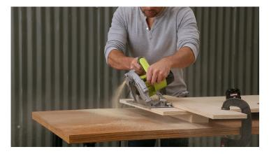
Adjust then the angle of the circular saw blade. To make the angled panels of the sled I adjusted the angle of the circular saw blade to the angles shown in the diagram.
