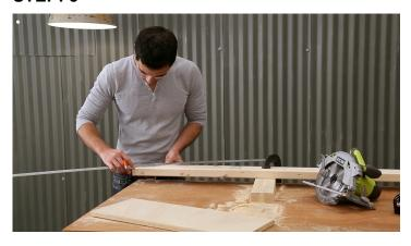
Make the beveled cuts. Clamp down a straight edge so that your cuts across the plywood are straight.
