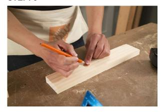
Mark the Handles. To center the handles and the end panels, mark 6 5/8. The handles need to be 4 inches wide. Mark 4 5/8 and 8 5/8. From the top edge, mark 1/2 inch and 1 1/4 inch. To round out the ends of the handles, use a penny as a template.
