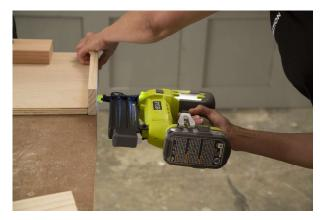
Assemble the Tray. Apply a small bead of wood glue along the edge of the base panel. Join one end board. Using your AirStrike, place 3-5 nails along the edge. Repeat these steps on the other end. Glue the left and right side of the hostess tray, and nail. Wipe off excess glue with a clean towel.
