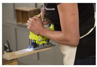
Cut out the Handles. Drill a small pilot hole in order to start cutting with your jig saw. Even up the cut from the back, if needed. Use fine sandpaper to smooth out sharp edges.
