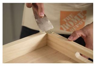
Fill Holes & Sand Tray Use wood filler to fill the nail holes, and use your sandpaper to lightly smooth out sharp edges. You're ready for decoration!
