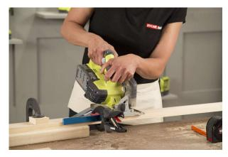
Cut Sides & End Panels. Cut 2 Sides & End Panels from the 1x3 using your Circular Saw. Side Board Cut: 18-1/2" x 21/2" (2) End Board w/ Handle Cut: 13-3/8" x 2-1/2" (2)
