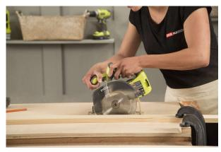
Cut the Base Panel. Measure the base panel and then cut it using your RYOBI Circular Saw. Base Panel Cut: 13-3/8" x 17"
