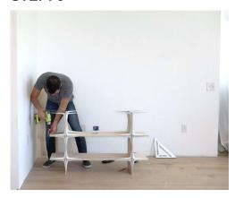
Screw the plywood to plywood If you want to save a little money and use fewer brackets you can just use brackets on the front face of the shelves and then use finish screws to screw the plywood to the plywood in the back.
