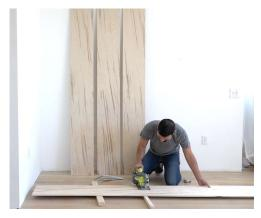
Cut the plywood to length I cut the plywood into the lengths shown in the drawing. I used my circular saw but this could also be done with a compound miter saw. I made my shelves 4 feet long with 11" tall vertical supports and 7" tall legs.
