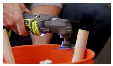
Wait 12 hours. Once the concrete has cured for at least 12 hours you can trim the legs with the Multi Tool. Just cut the legs using the edge of the bucket as a guide. You can also use the multi tool to sand the legs.
