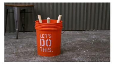
Place the legs. Once the concrete has settled, place the legs in the bucket. Stick the legs about 1 ½" past the surface of the concrete and let them rest against the sides of the bucket.
