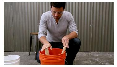
Shake out the bubbles. Mixed concrete has air bubbles trapped inside. Shake and tap the bucket to bring the bubbles to the surface.
