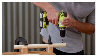
Drill holes in the legs. Drill  $\frac{1}{4}$ " diameter holes about one inch from one end of the dowels.
