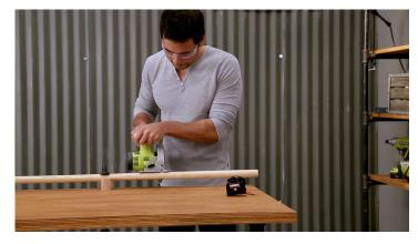
Cut the legs. Cut the 48" dowel into three pieces 16" long each.
