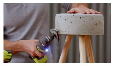
Sand the edges. The concrete has not yet fully hardened and is pretty easy to work with. 120 grit sand paper can be used to smooth the edges.
