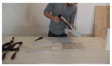
Glue the pieces together. I used liquid nails to glue the pieces together. I didn't want to have to clean off lots of adhesive off the exterior so tried to be careful not to use too much adhesive. Gorilla 2-part epoxy also works well but is a bit more expensive. Make sure to even spread the adhesive on the edges and then wipe off any exterior adhesive on the outside.
