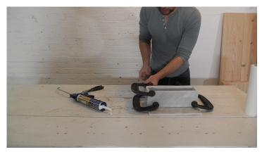
Clamp it together. For the first planter I used C-clamps and screwed them a little too tight. I caused a small crack in one of the planters. The crack was small so I was able to seal it from the inside with liquid nails. For the 2nd planter I used rubber bands to hold it together and that worked really well.
