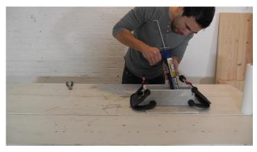
Let the glue dry. I let the glue dry overnight before removing the clamps and testing to see if the planters held water. If they leak simply caulk the interior seams with liquid nails or construction adhesive.
