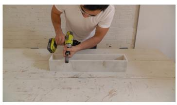
Sand the edges. The edges for one of the planters were a bit sharp so I put a drum sander in my drill and rounded them down
